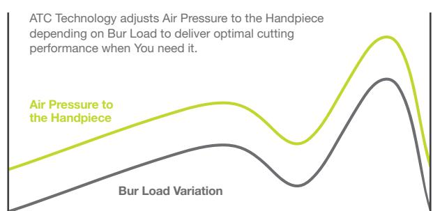
A sensor in the coupler picks up the frequency of vibrations caused by the speed of the rotating bur. When the bur encounters a higher load that normally causes a decrease in speed, a signal from the control source increases air pressure and thereby the rotation of the turbine, thus maximizing cutting efficiency. The opposite occurs when the bur encounters a lighter load.
